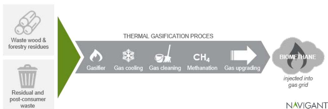
Figure 8 Schematic overview of the thermal gasification process
